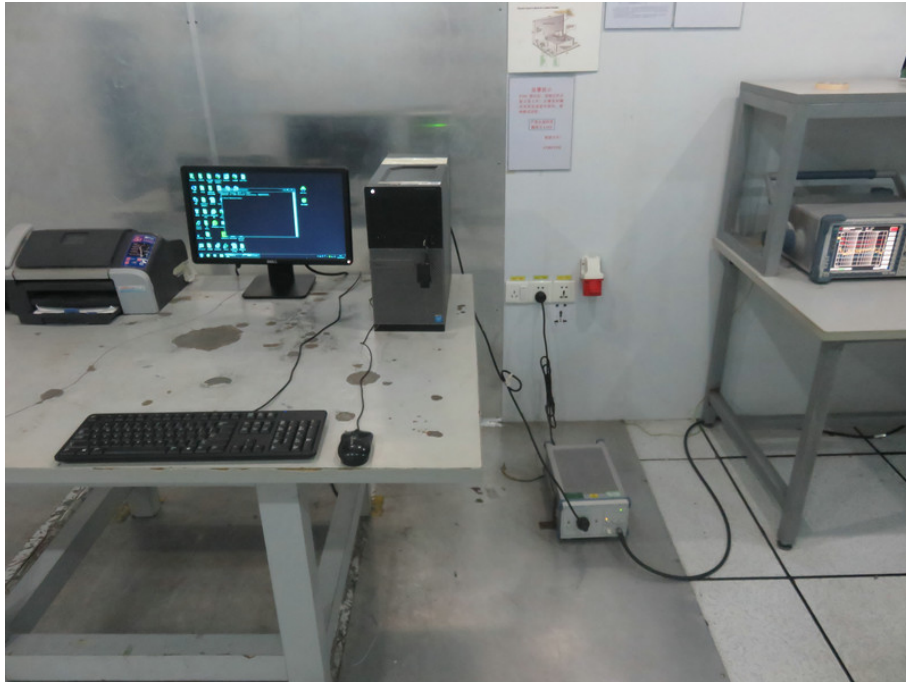
1. Photo of Power Line Conducted Emission Measurement
