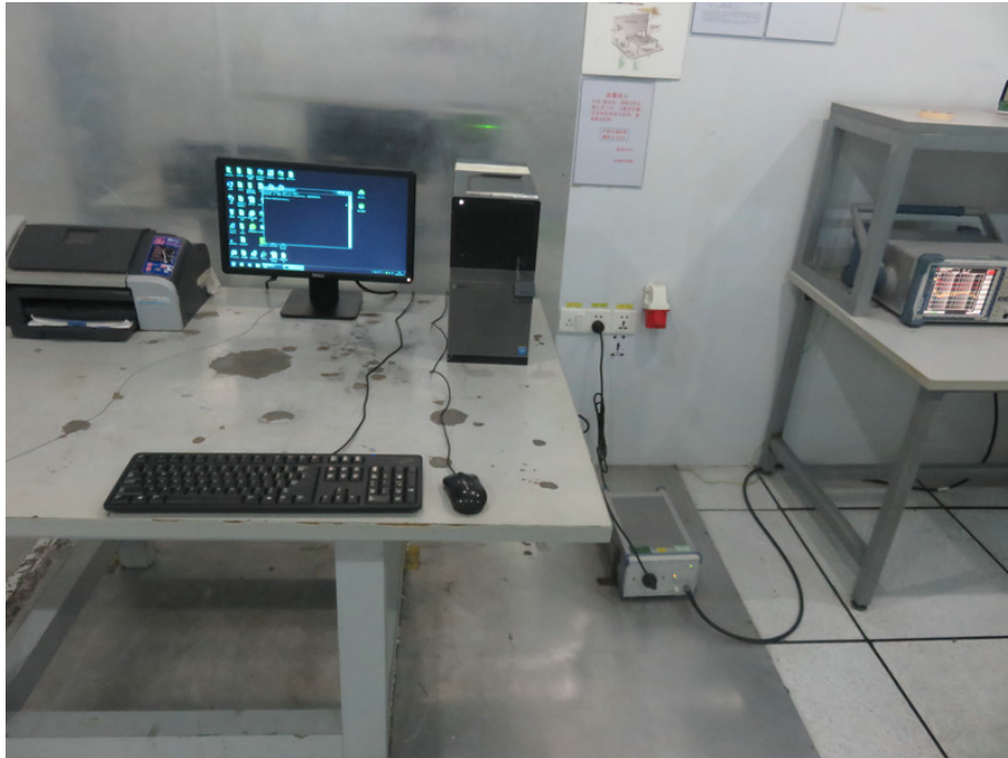
1. Photo of Power Line Conducted Emission Measurement
