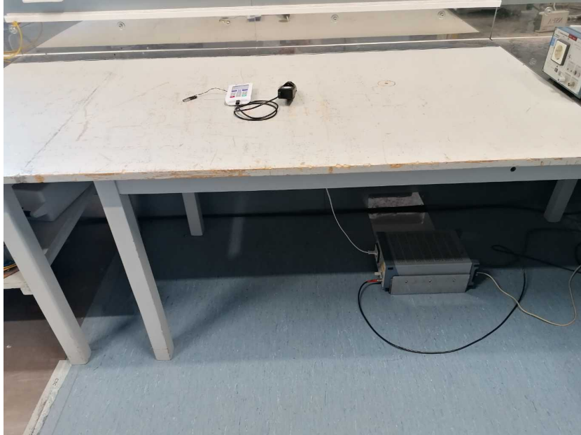
Photo 11: AC conducted emission test setup
