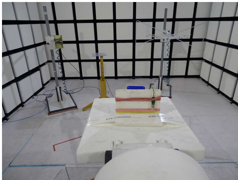
Photo 4: EUT at the anechoic chamber
