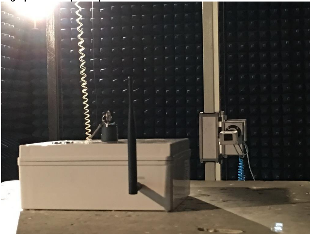
Photograph 4: Set-up for Spurious Emissions of 18 – 26.5GHz
