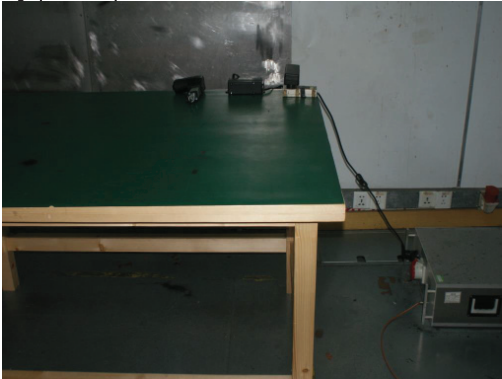
Photograph 5: Set-up for Conducted Emission
