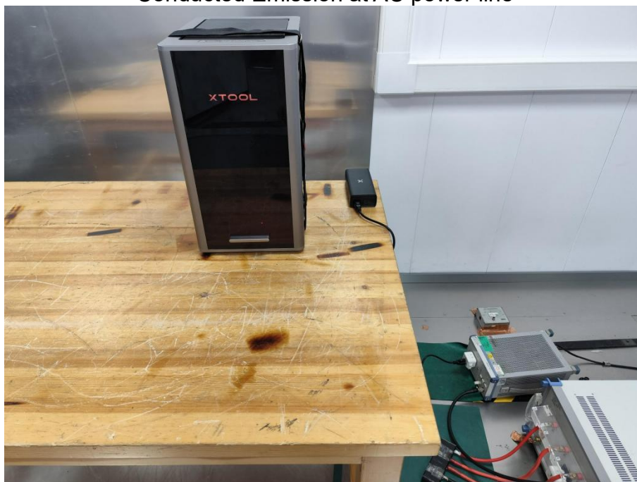
Conducted Emission at AC power line
