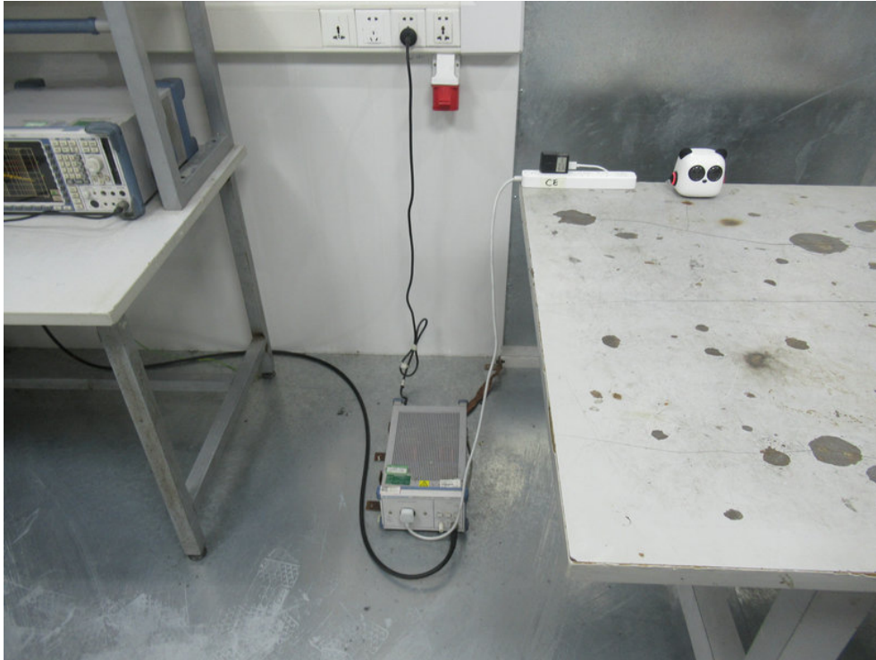
Photo of Conducted Emission Measurement
