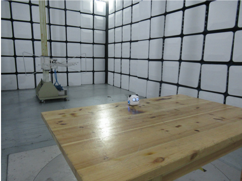
Photo of Radiation Emission Test
