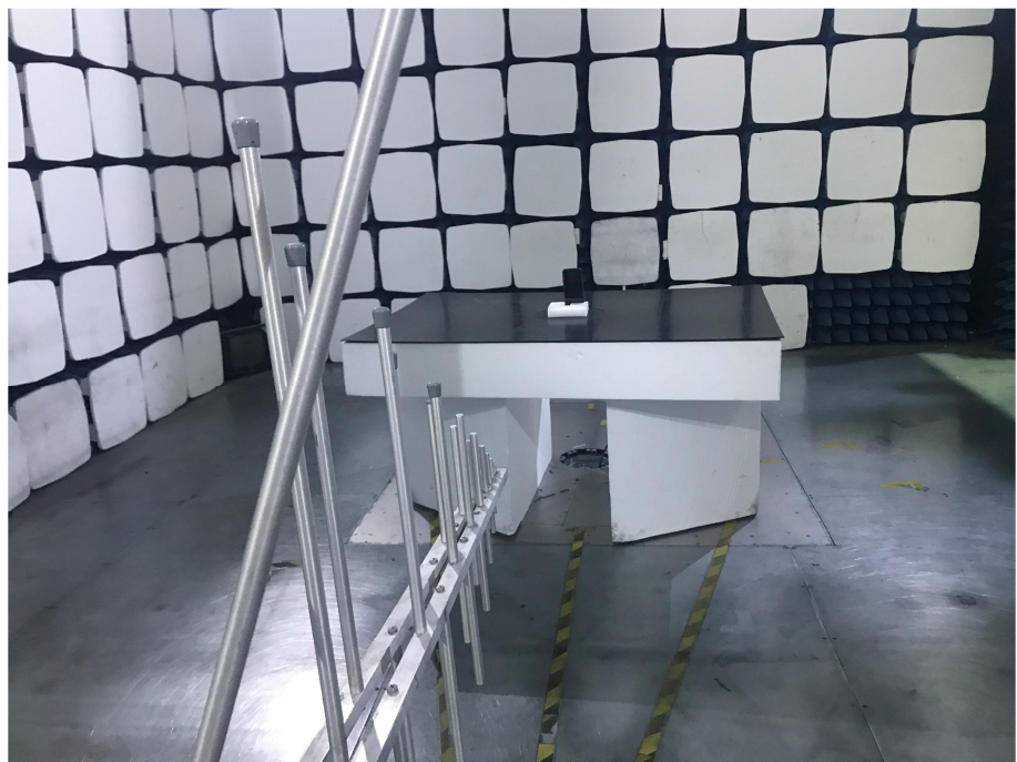
Radiation Emission Test Setup (30MHz to 1GHz)
