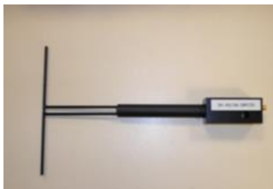
Figure 1 – MVG COMOSAR Validation Dipole
