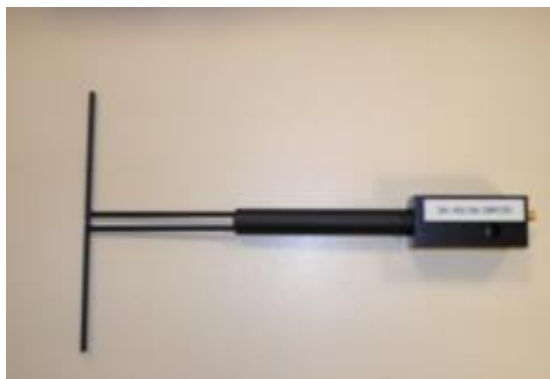
Figure 1 – MVG COMOSAR Validation Dipole
