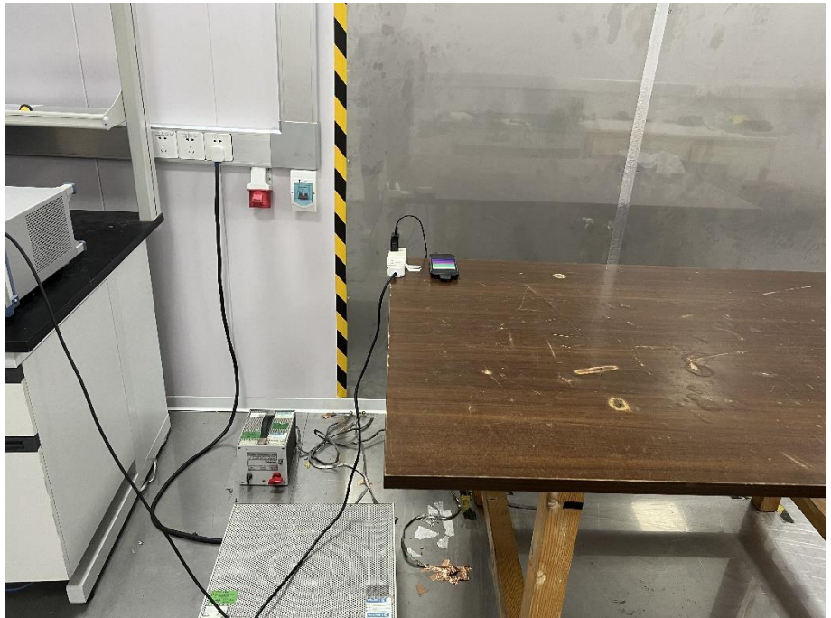
Conducted Emission Test Setup
