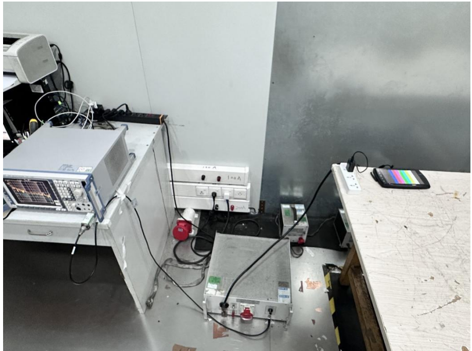
Conducted Emission Test Setup
