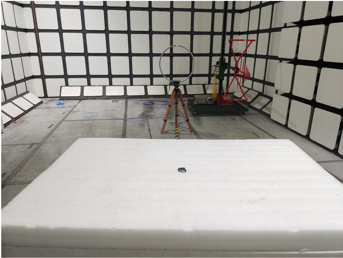
Radiated Emissions View (Below 30MHz)
