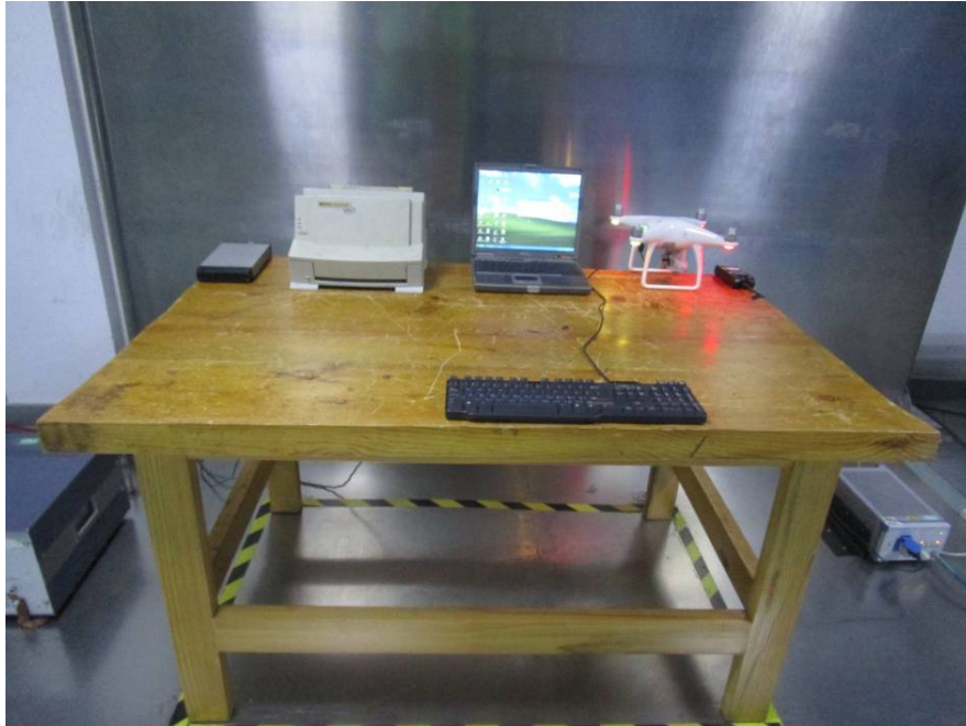
Conducted Emission – Front View (Downloading Mode)
