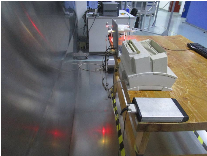
Conducted Emission – Side View (Downloading Mode)
