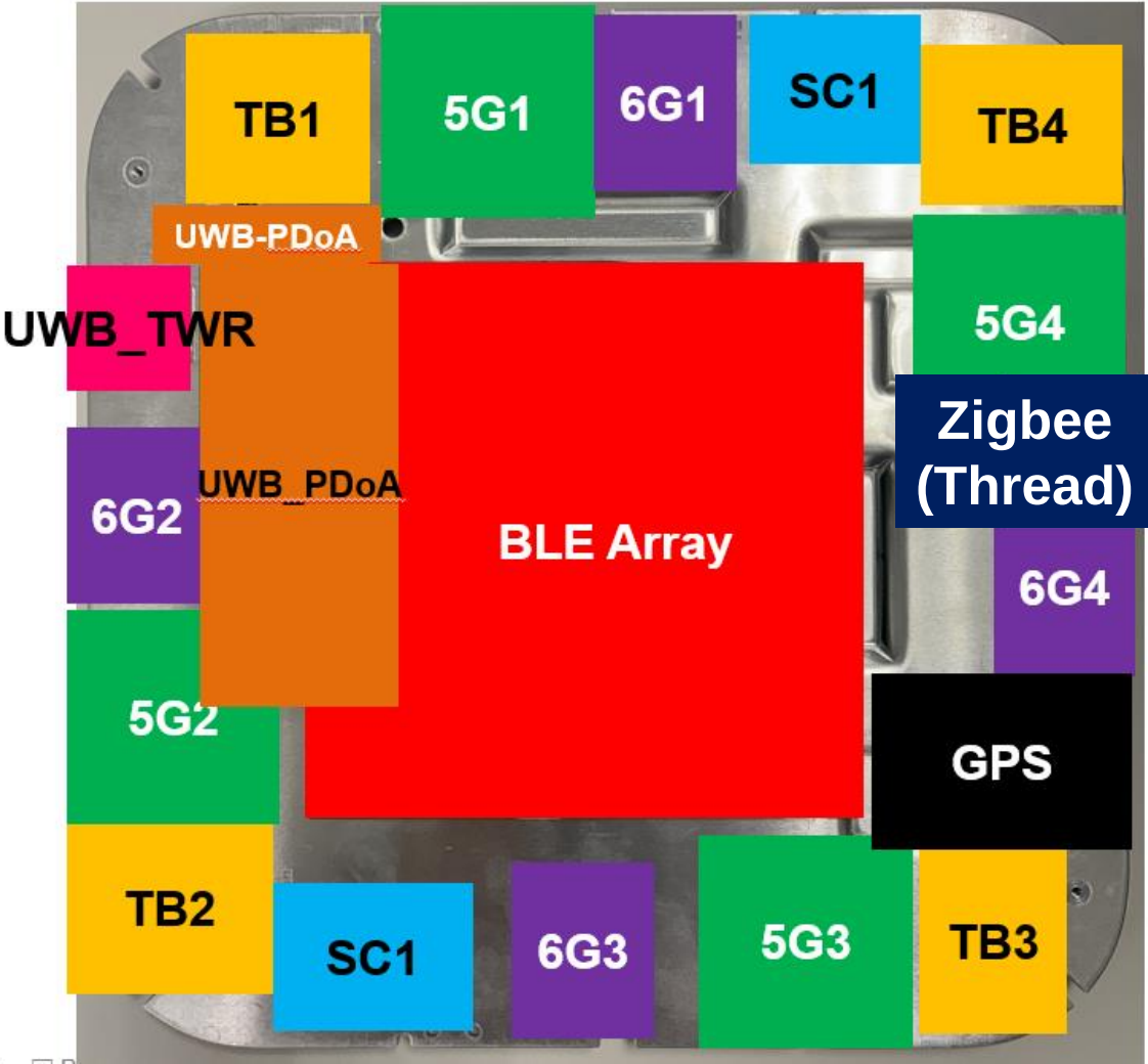
Antenna Plate: 246x246mm
