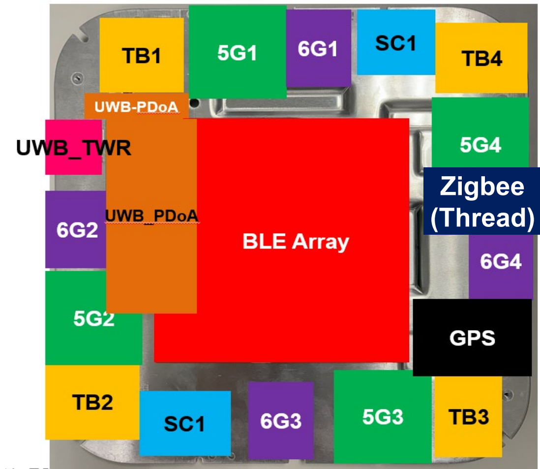
Antenna Plate: 246x246mm
