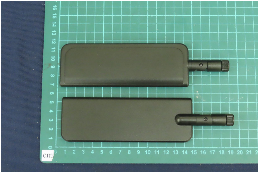
(9) EUT Photo_Apex TG.30 5G/4G Terminal Antenna: Hinged SMA(M) / TAOGLAS TG.30.8113
