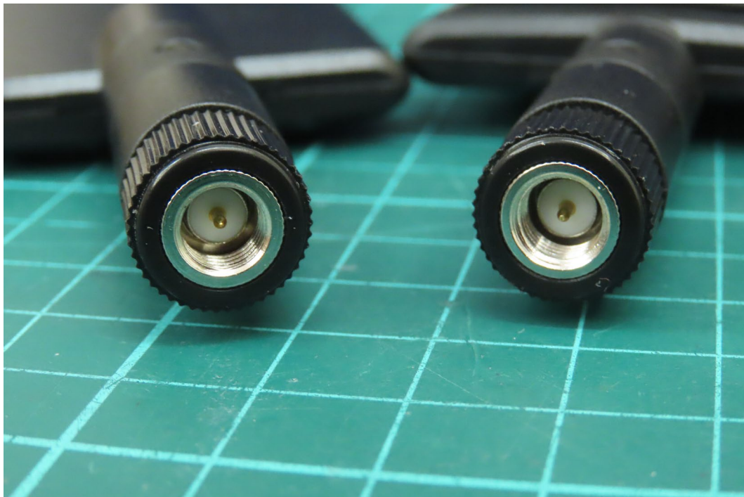
(10) EUT Photo_Apex TG.30 5G/4G Terminal Antenna: Hinged SMA(M) / TAOGLAS TG.30.8113
