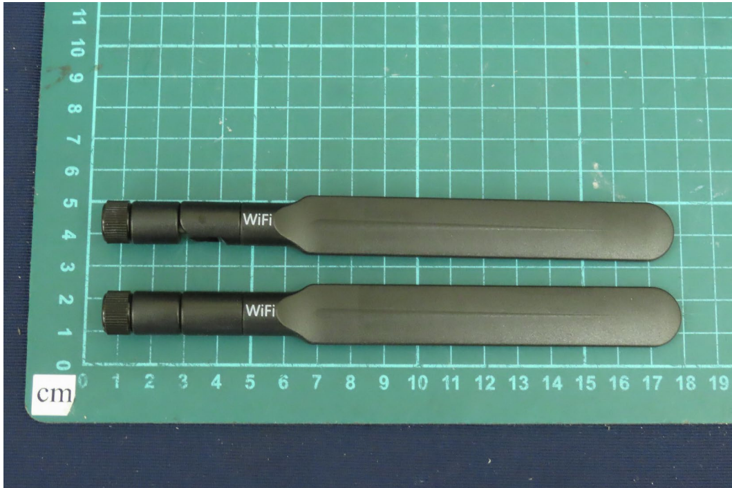
(7) EUT Photo_WIFI DUAL-BAND SMA ANTENNA:Teltonika / PR14RD35
