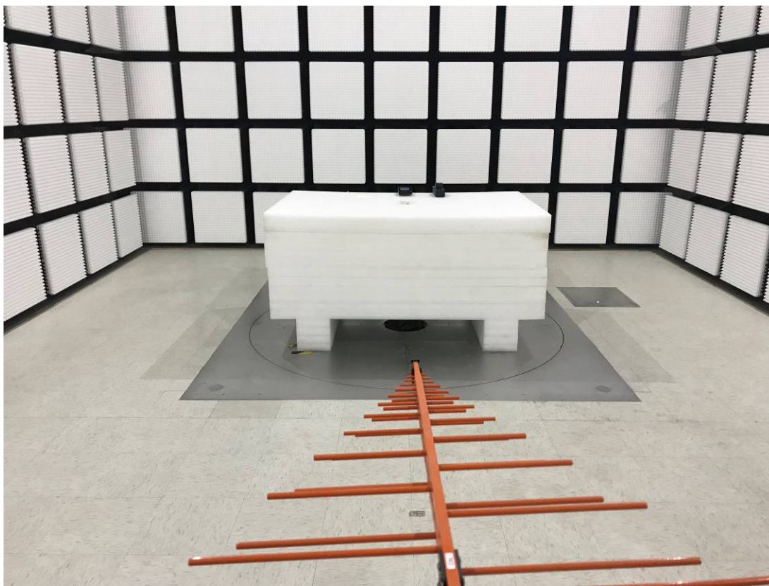
Radiated Emission Below 1G rear View-Adapter
