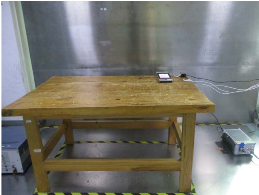
Conducted Emissions – Front View(PoE Adapter supply)
