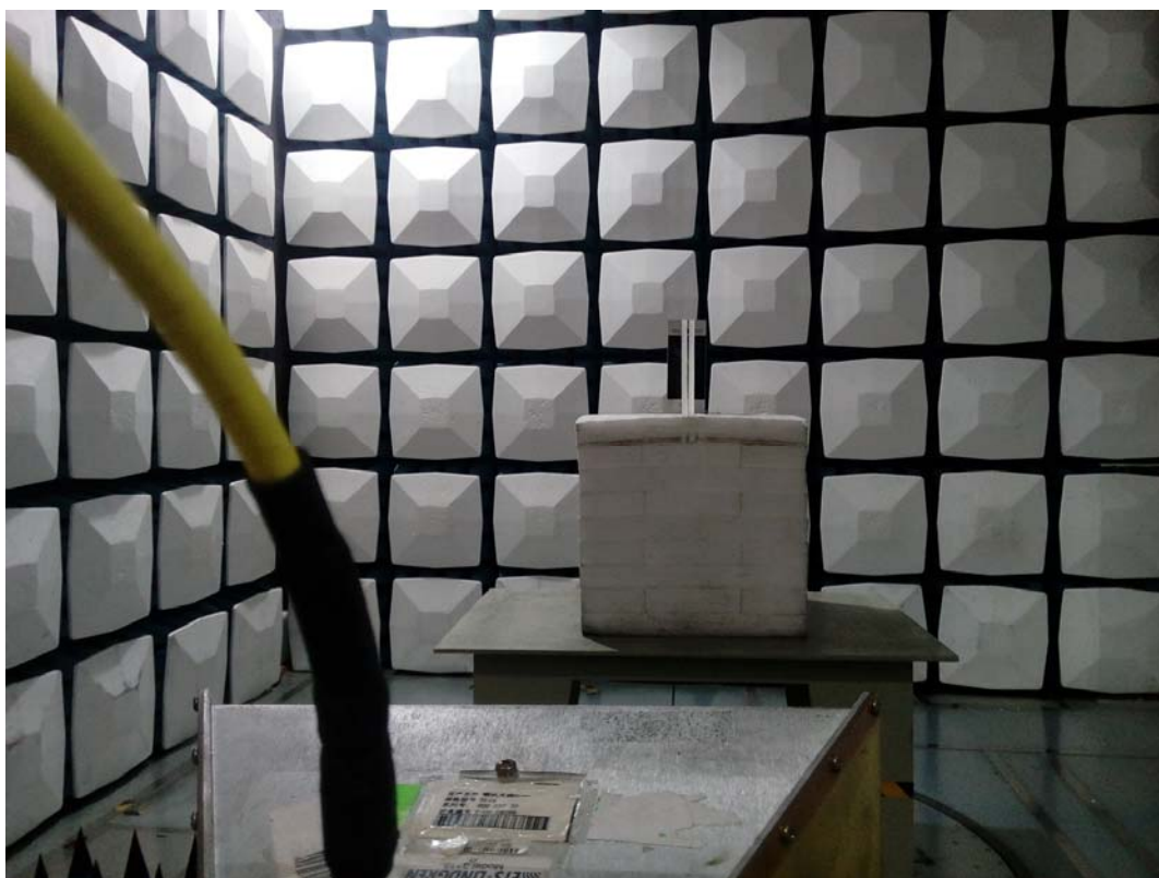
Radiated Emission Above 1GHz View
