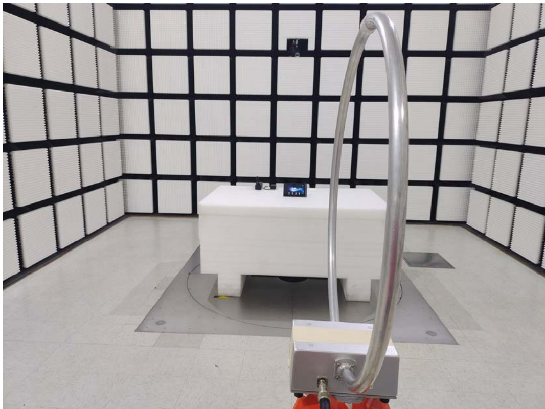
9kHz~30MHz _ Radiated Emission View - Perpendicular _POE
