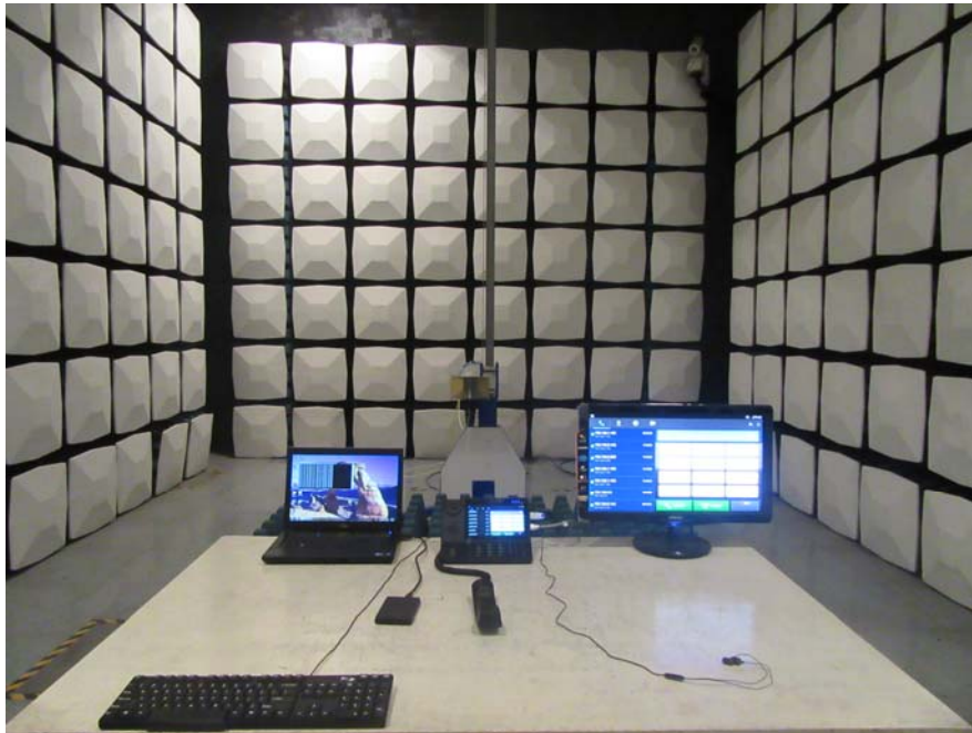
Radiated Emission - Front View (Above 1 GHz)
