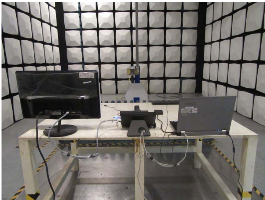
Radiated Emission - Rear View (Above 1 GHz)
