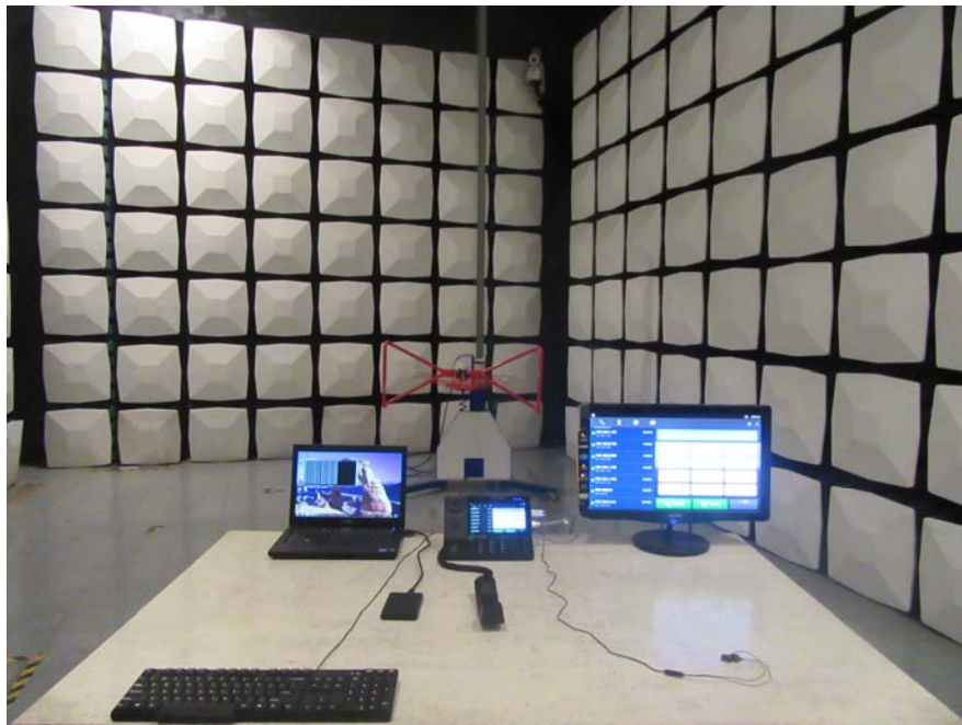
Radiated Emissions - Front View (Below 1GHz)
