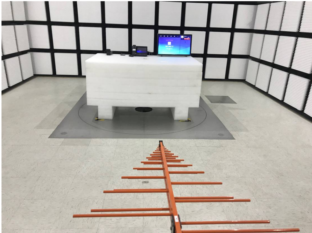
Radiated Emissions Below 1G rear View –AC/DC Adapter
