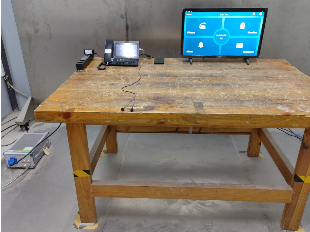
Conducted Emissions Side View - AC/DC Adapter
