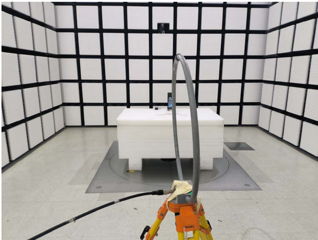
Radiated Emission Below 1GHz View Ground-parallel
