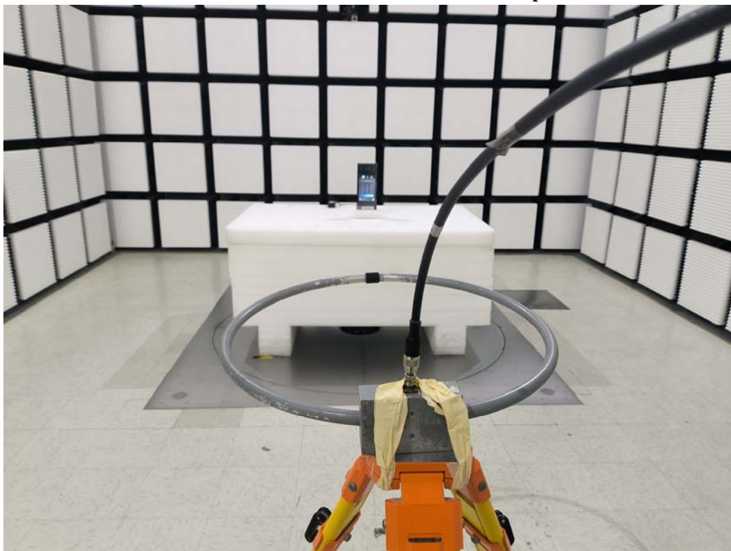
Radiated Emission Below 1GHz View Ground-parallel
