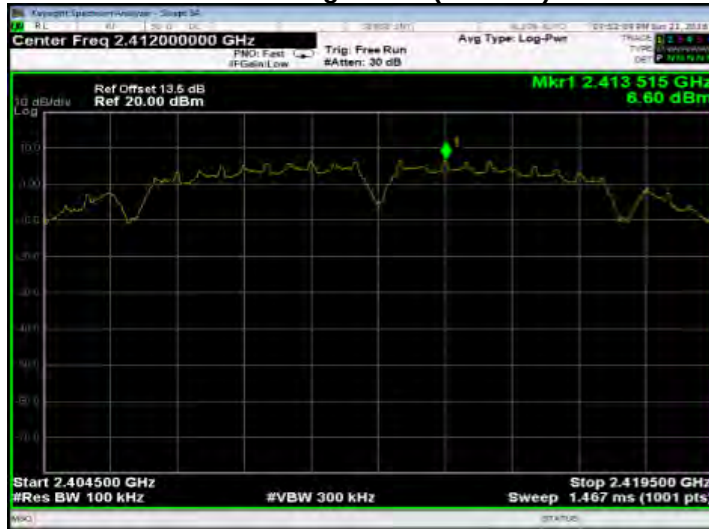
802.11b PSD for Bandedge Limit(CH-High)
