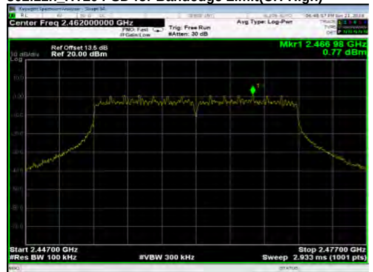
802.11n HT20 PSD for Bandedge Limit(CH-High)
