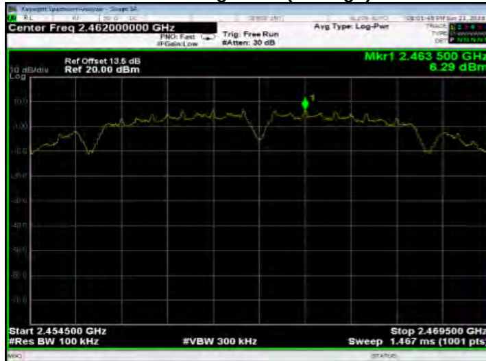
802.11g PSD for Bandedge Limit(CH-Low)
