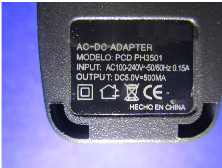
EUT – Adapter Label View
