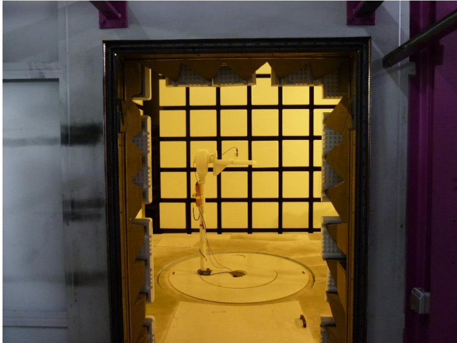
Photo 1: EUT at the anechoic chamber
