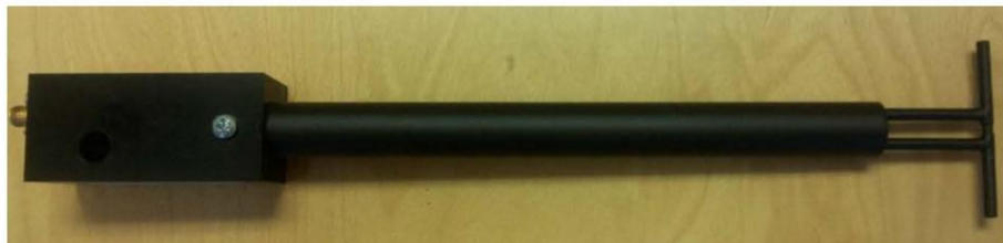
Figure 1 – MVG COMOSAR Validation Dipole
