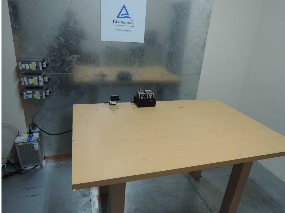
Photograph 4: Set-up for for Mains Conducted testing Front
