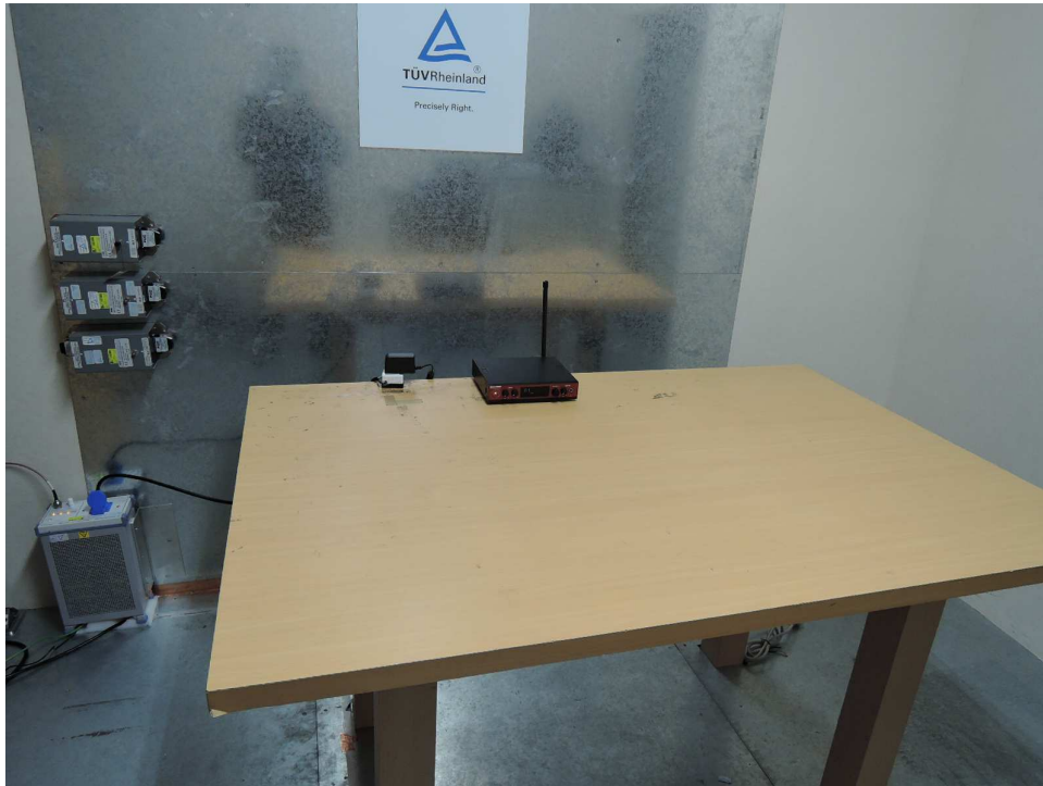
Photograph 6: Set-up for for Mains Conducted testing Front
