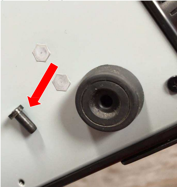
(Pressure fit plug removed from the MV-ALS-STFM foot.)
