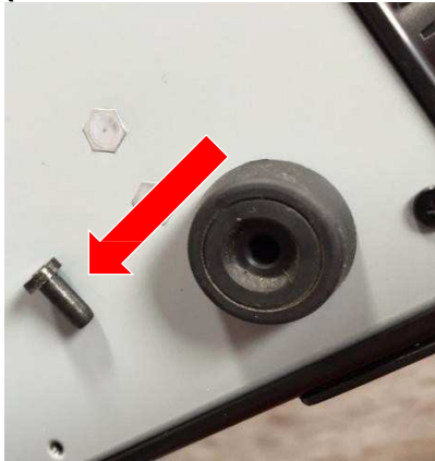
(Screw Removed from the MV-ALS-STFM Foot.)
