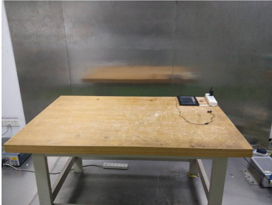
Conducted Emissions - Front View
