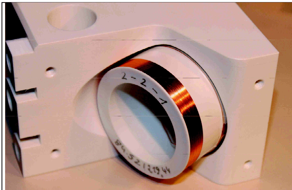
Figure 23: transmitter coils in Schiff5 mounted
