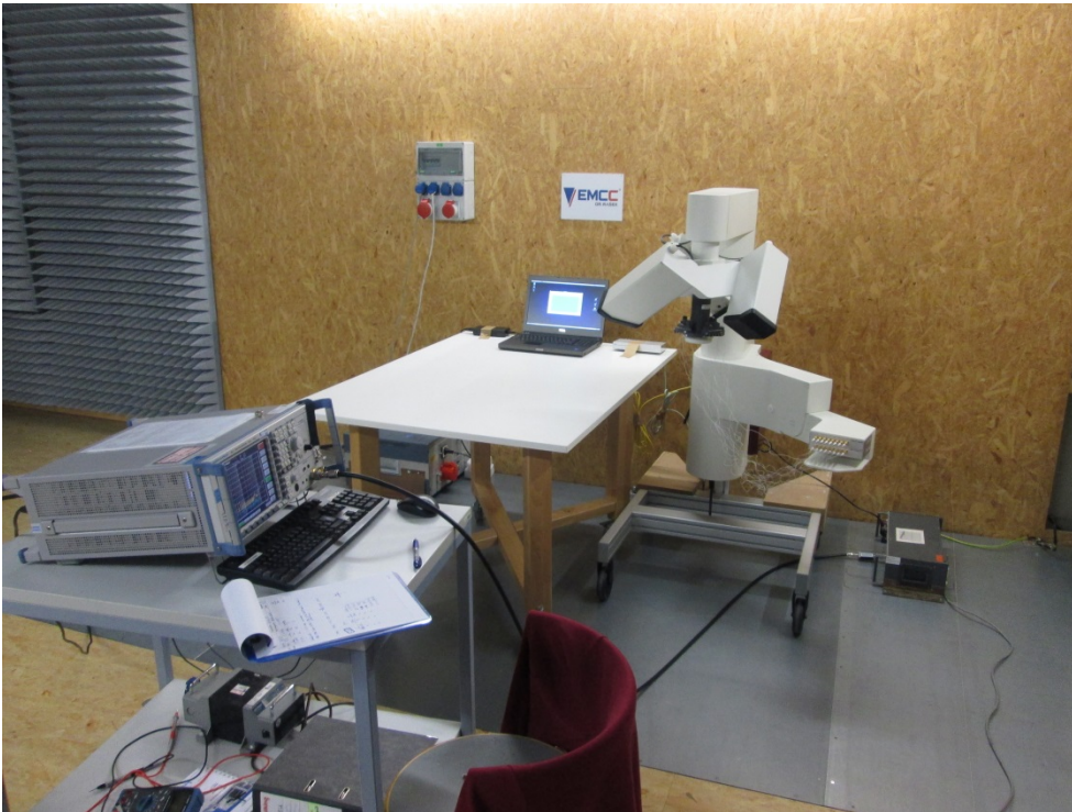
Photo A1-1: Conducted emissions measurement
