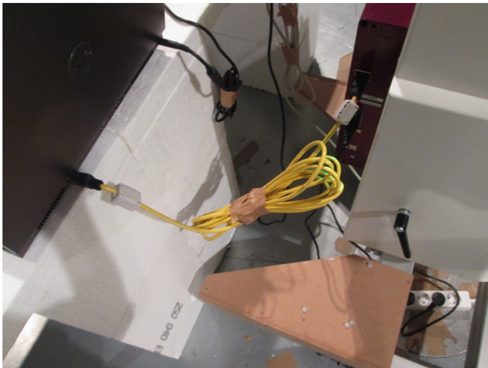
Photo A3-1: Modification 1, ferrites at Ethernet cable
