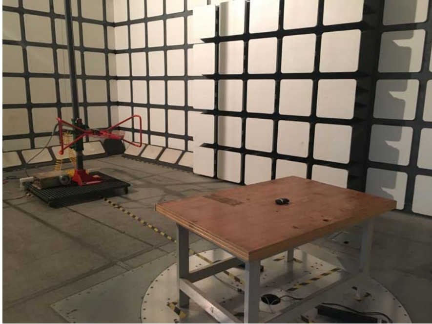
Radiated Emissions View
