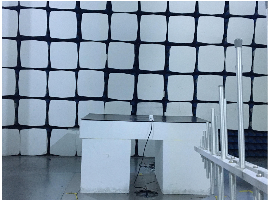
Radiation Emission Test Setup (30MHz to 1GHz)
