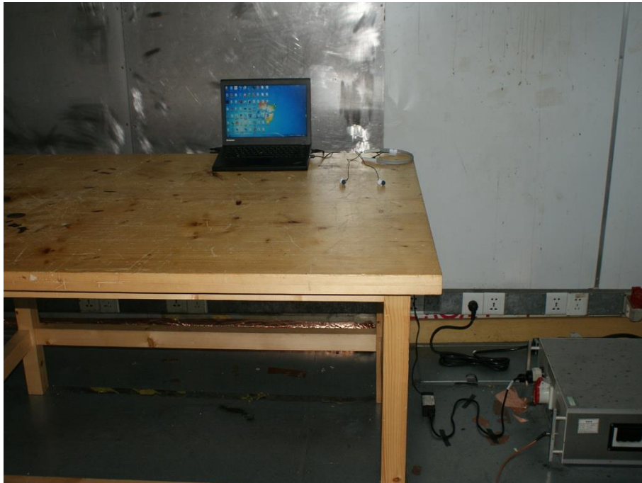
Photograph 1: Set-up for Conducted Emission on AC Mains
