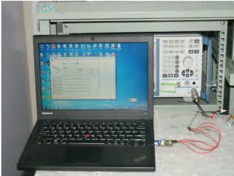
Photograph 2: Set-up for Radiated Spurious Emission (9kHz ~ 30MHz)
