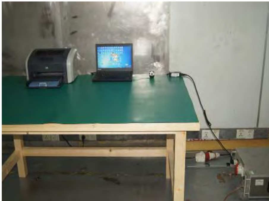
Photograph 6: Set-up for Conducted Emission
