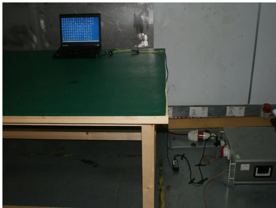
Photograph 4: Set-up for Conducted Emission on AC Mains
