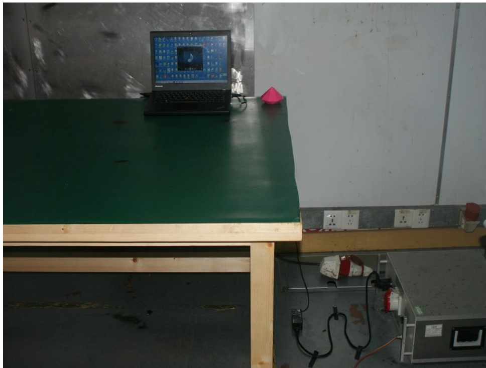
Photograph 6: Set-up for Conducted Emissions
