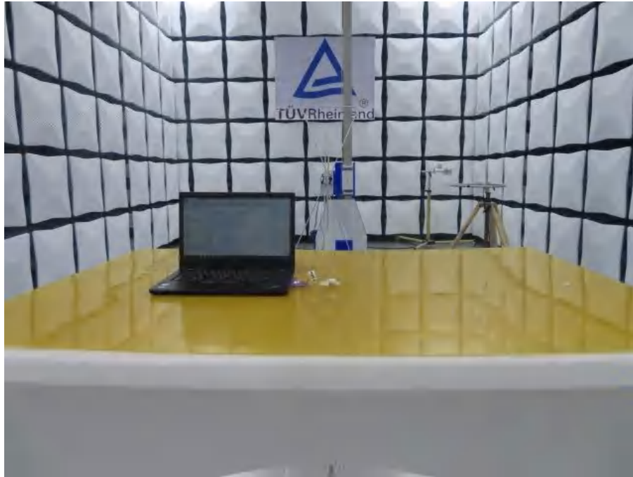
Photograph 1: Set-up for Radiated Spurious Emission, 30MHz ~ 1GHz
