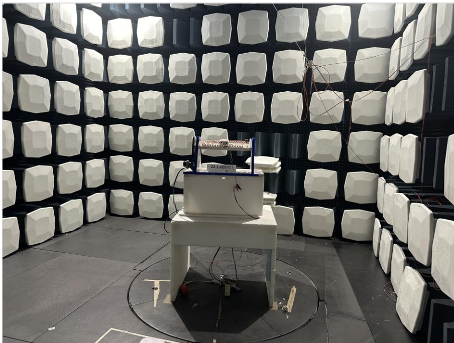
Photograph 9: EUT test setup in the fully anechoic chamber, overview_EUT elevation 0°
