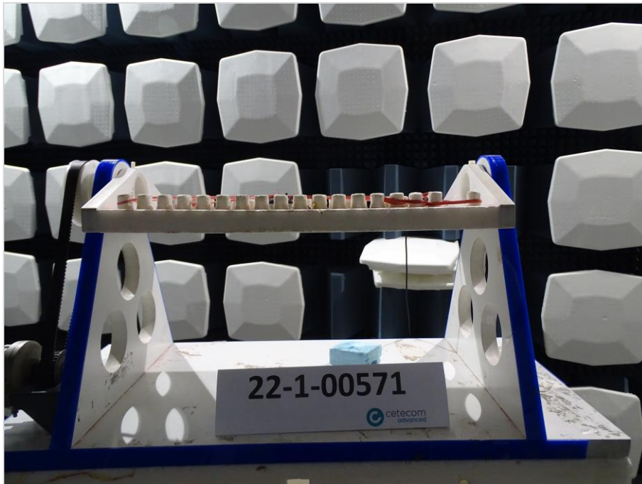
Photograph 9: EUT test setup in the fully anechoic chamber, close up view_EUT elevation 90°
