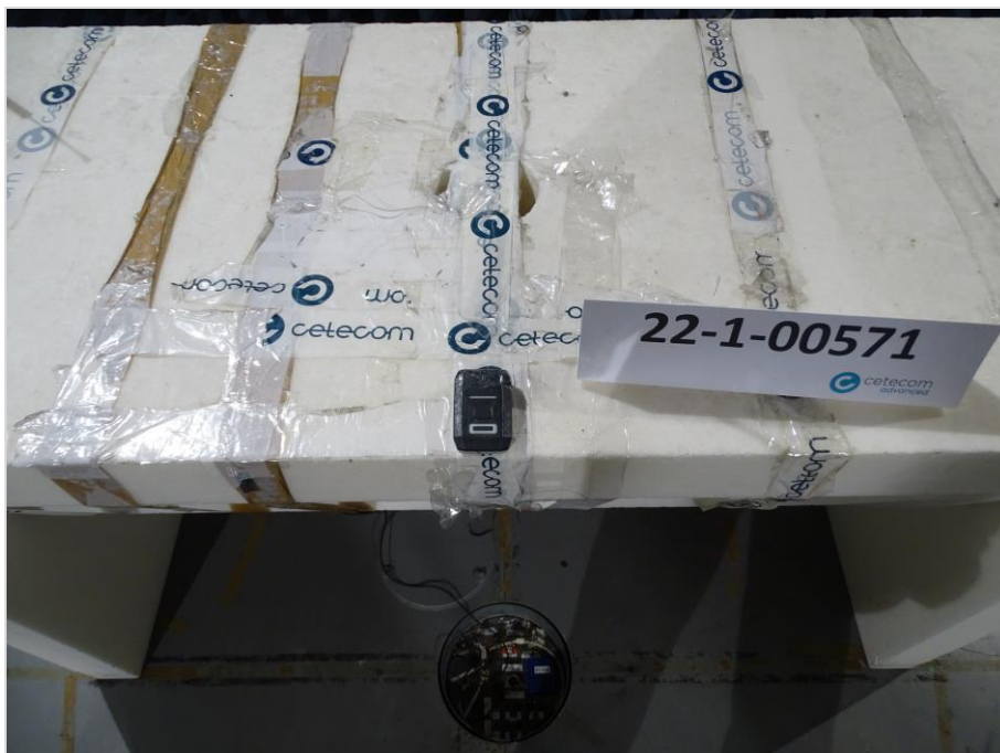
Photograph 5: EUT test setup in the semi anechoic chamber, close up view_EUT elevation 90°
