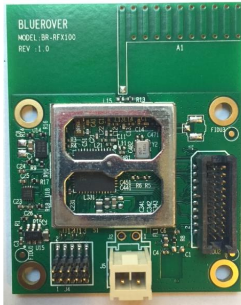
Internal View of EUT (No U.FL) - Front
