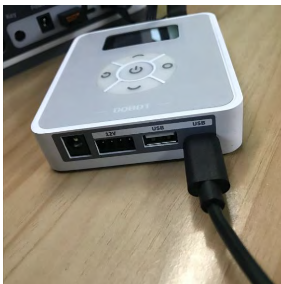
Figure 2.5 Connect Magician Lite to the electrical outlet
