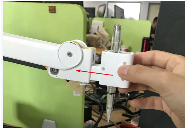
Figure 5.34 Install a writing and drawing kit
