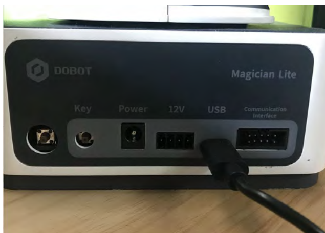
Figure 2.2 Connect Magician Lite to your computer
