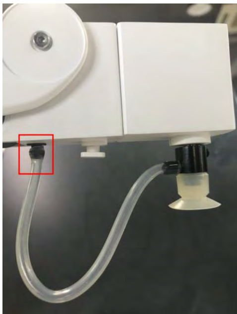
Figure 5.10 Install an air tube
