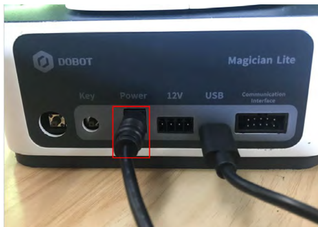
Figure 2.3 Connect Magician Lite to the electrical outlet
