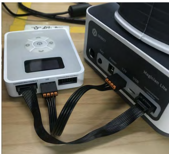
Figure 2.4 Connect Magician Lite and Magic Box
