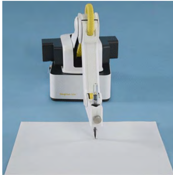
Figure 5.51 Adjust the position of the pen nib
