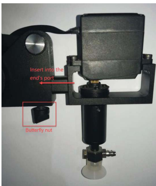
Figure 5.8 Install a suction cup kit
