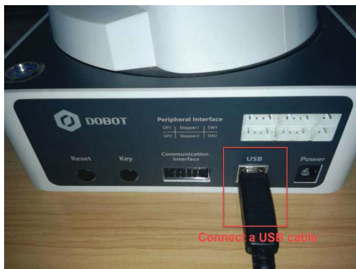
Figure 2.2 Connect the Dobot Magician to your computer
