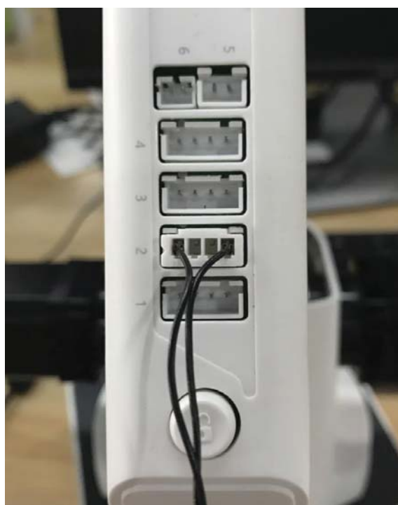
Figure 5.169 Insert the cable of the auto-levelling
