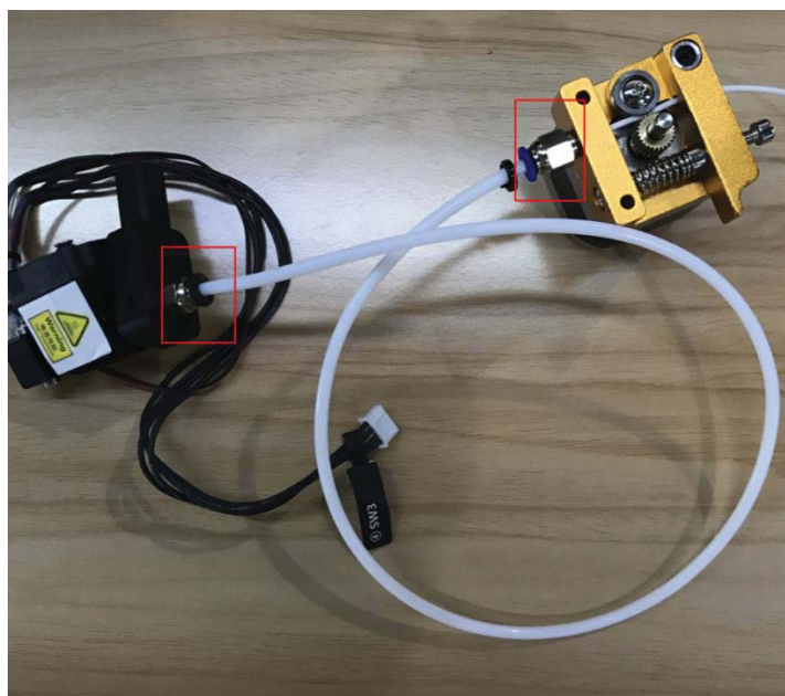
Figure 5.119 Connect extruder and hot end
