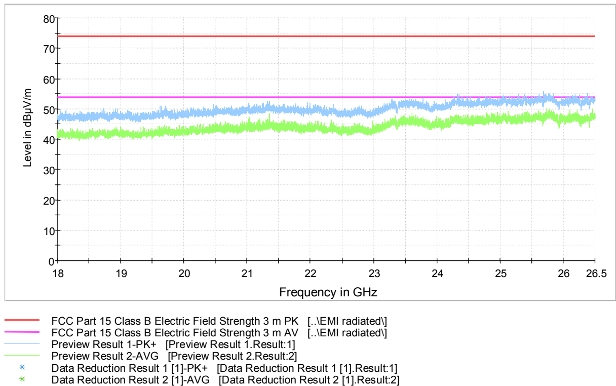
Figure 13. Measured curve with peak and average detectors (Low channel).
