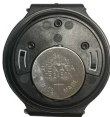
Figure 11: MBD-2 Correctly Installed Battery Position
