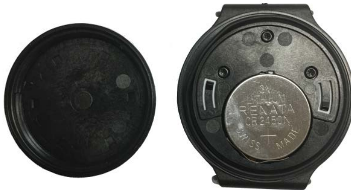
Figure 8: MBD-2 Battery Cover Removed
