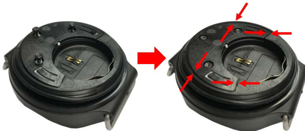
Figure 19: Installing the Internal Battery Cover
