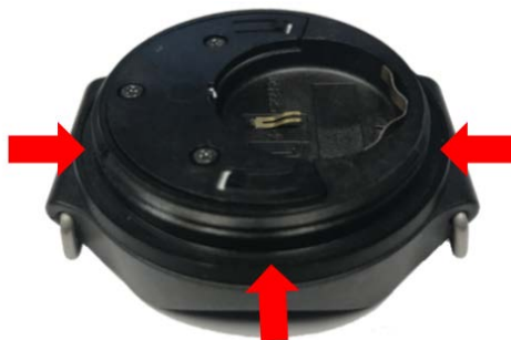
Figure 16: MBD-2 without O-Ring and Inspection
