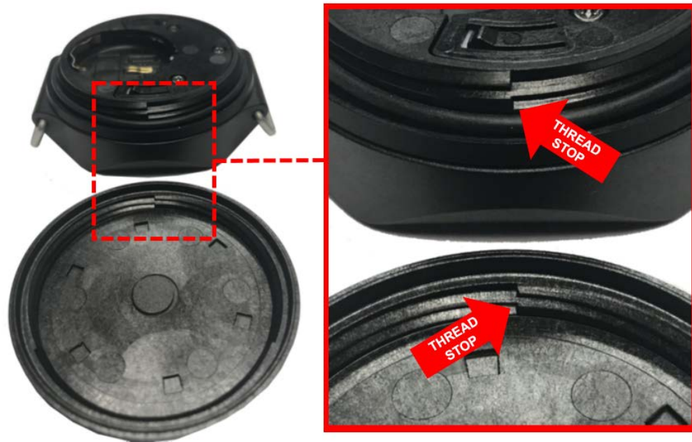
Figure 12: MBD-2 and Main Battery Cover Thread Stops
