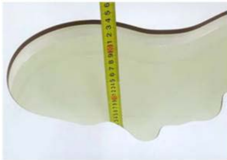
Photograph of the depth in the Head Phantom (1900MHz)
